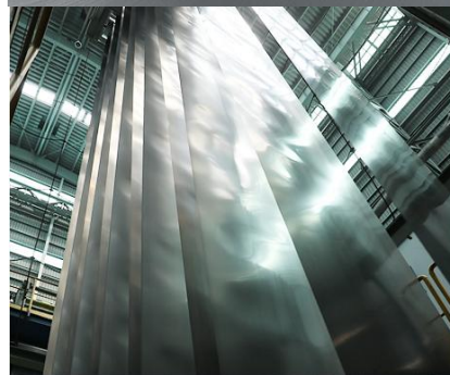
step3 ENTRY ACCUMULATOR SECTION To compensate for the down time before the welding process, strip is accumulated at the entry section.
